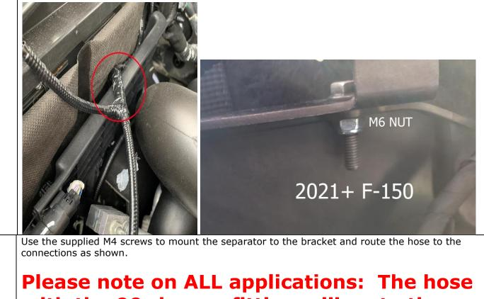
Please note on ALL applications: The hose with the 90-degree fitting will go to the PCV valve. The hose with the 45-Degree fitting will go to the intake manifold.
